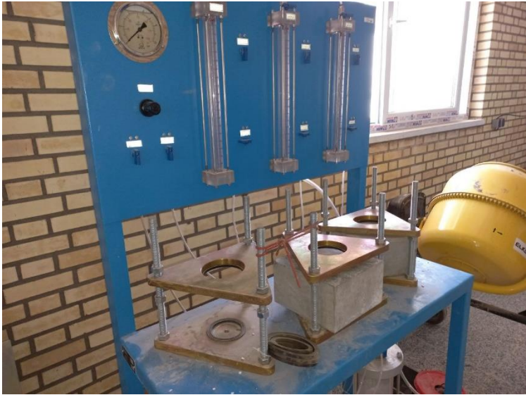
Figure 17 An image of the permeability test apparatus
