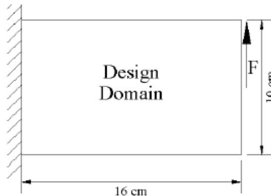
Figure 2. The cantilever beam topology optimization problem under the load ( F=500 N) [9].
