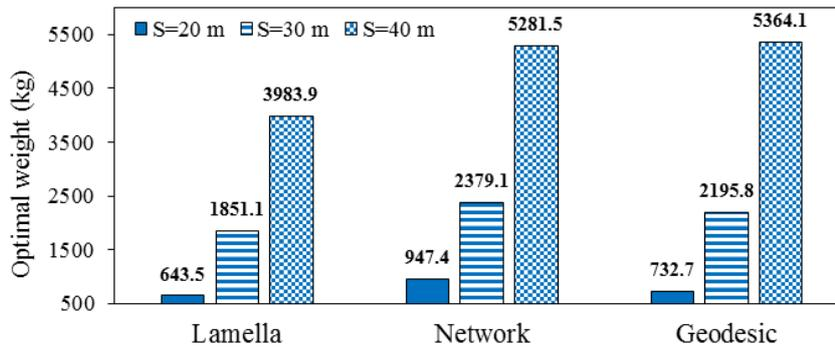
Figure 5. Optimal weight of domes for  $Q = 375 \text{ kg/cm}^2$
