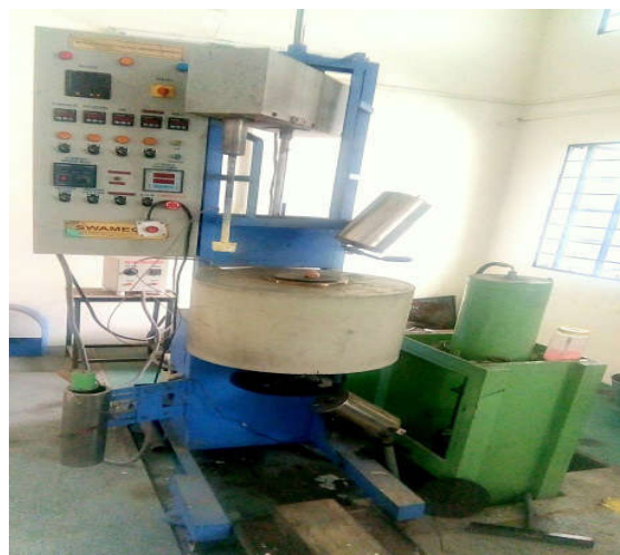
Fig. 1. Squeeze casting machine setup
