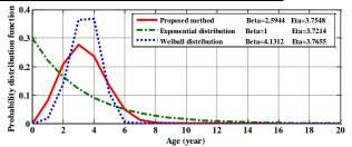
Fig. 4 Probability distribution of the time between failure for the OLTC, MTBF=3.3548.
