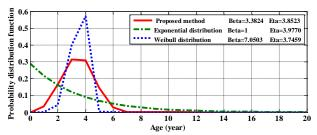
Fig. 8 Probability distribution of the time between failure for the tank and accessories, MTBF=4.5023.
