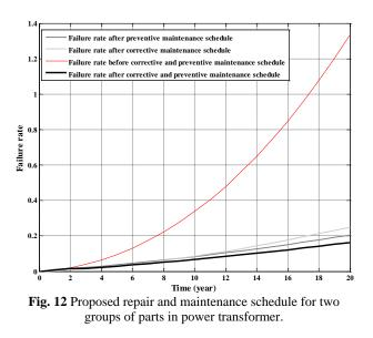
Weibull distribution that obtained from the actual failure data shows that the failure rate characteristic of each component is time-dependent. Therefore, by using the proposed method results, a preventive maintenance program can be scheduled for higher significant components that reduce the risk of forced outages of power transformers at various voltage levels.
