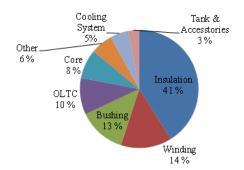
Fig. 2 Share of failures percent in power transformers components [8].
