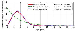
Fig. 3 Probability distribution of the time between failure for the insulation, MTBF=3.4074.
