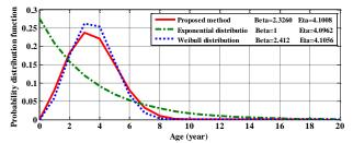
Fig. 9 Probability distribution of the time between failure for the core, MTBF=4.5823.
