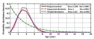
Fig. 7 Probability distribution of the time between failure for the cooling system, MTBF=4.1280.
