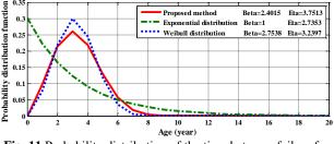
Fig. 11 Probability distribution of the time between failure for transformer, MTBF=3.9751.
