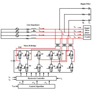
Fig. 4 Three H-bridge based DSTATCOM.
