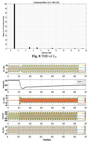
Fig. 10 Performance of three-pole voltage source converter with T-connected transformer based DSTATCOM.
