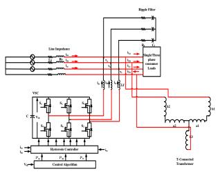
Fig. 3 Three-pole voltage source converter with T-connected transformer based DSTATCOM.
