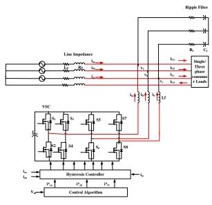
Fig. 2 Four-pole voltage source converter based DSTATCOM.
