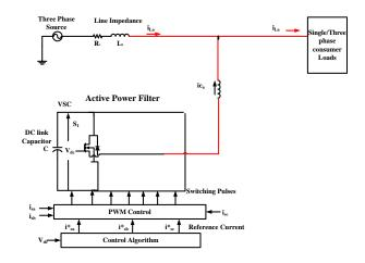
Fig. 1 Pictorial view of DSTATCOM topology.
