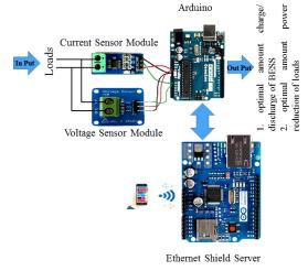
Fig. 3 The proposed implementation of the load management system for each of the consumers.
