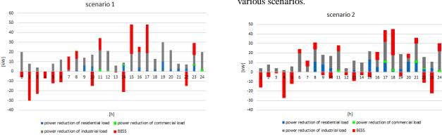
Fig. 6 Power of BESS and power of the consumers in scenario 1.
