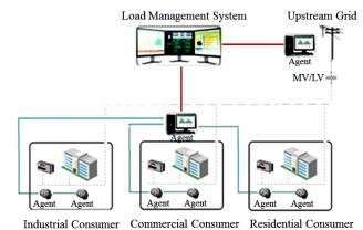
**Fig. 1** Micro-grid structure based on agents.
