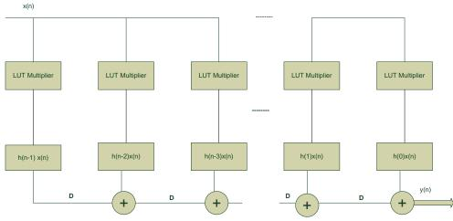
Fig. 9 Modified transposed FIR filter structure.
