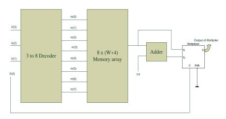
Fig. 2 Proposed EMS-LUT multiplier for 4-bit input.
