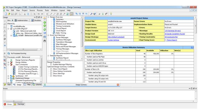
Fig. 7 Device utilization summary of OMS multiplier with 64-bit input.
