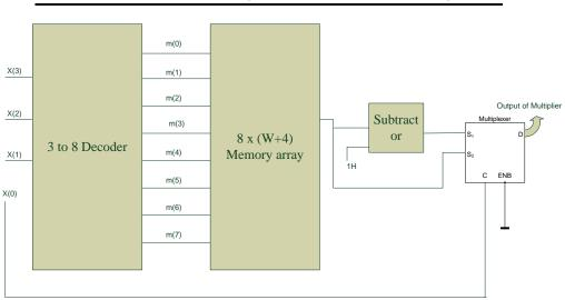
Fig. 4 Proposed modified OMS-LUT multiplier for 4-bit input.
