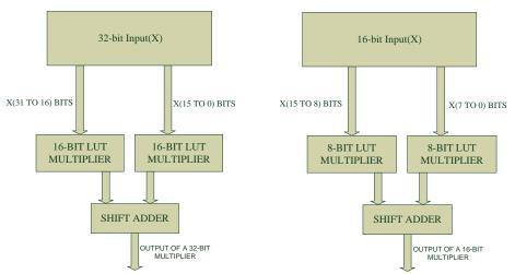
Fig. 6 Block diagram of 32-bit and 16-bit LUT-based multiplier.
