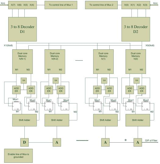
Fig. 10 Transposed FIR filter structure using the proposed EMS-LUT multiplier.
