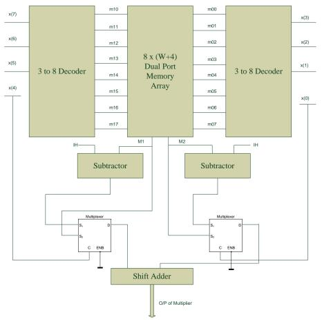
Fig. 5 Proposed modified OMS-LUT multiplier for 8-bit input.
