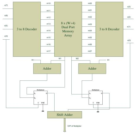
Fig. 3 Proposed EMS-LUT multiplier for 8-bit input.
