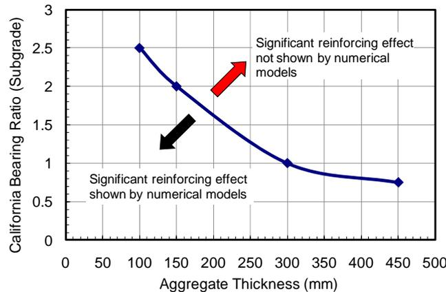
**Fig. 11** Geogrid-reinforcing threshold curve
