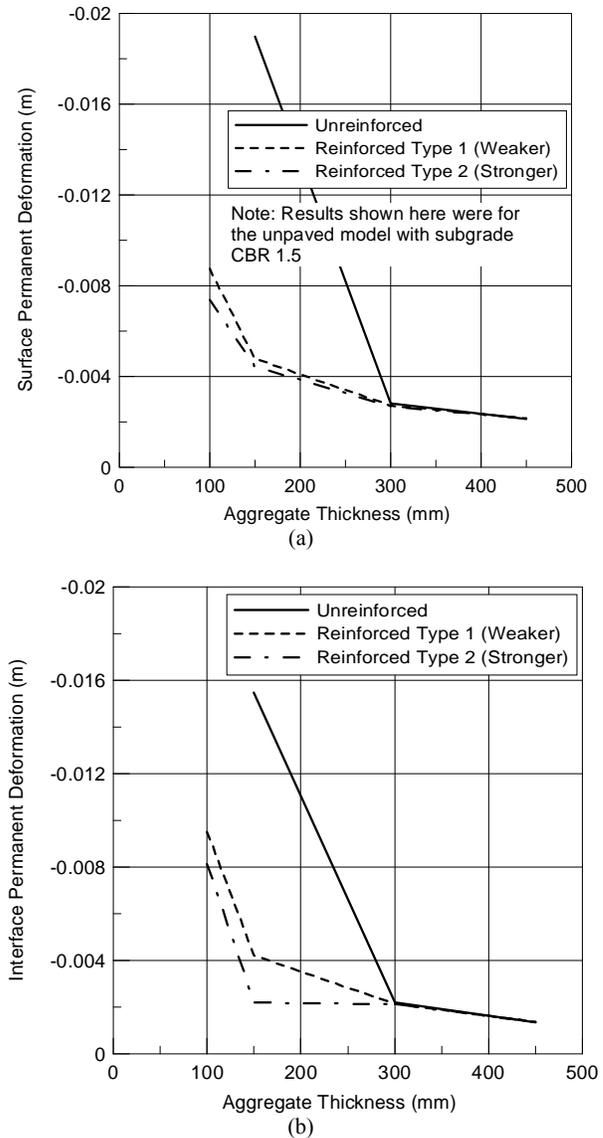
**Fig. 9** Plastic deformation V.S. aggregate thickness at (a) surface and (b) interface
