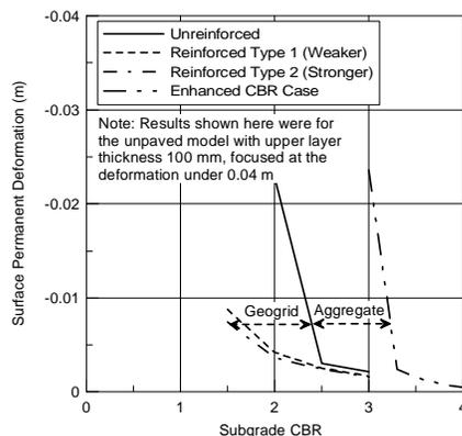
Fig. 13 Enhanced subgrade CBR analysis for aggregate layer thickness of 100mm
