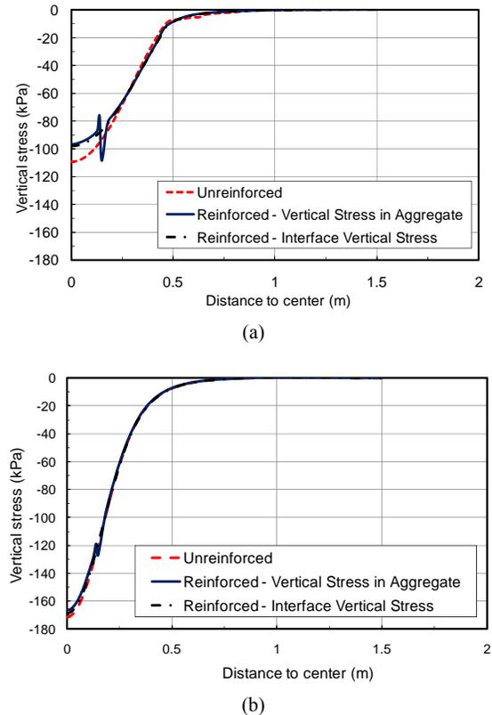
**Fig. 8** Vertical stress distribution at the top of the subgrade layer for subgrade (a) CBR 0.75 (b) CBR 3
