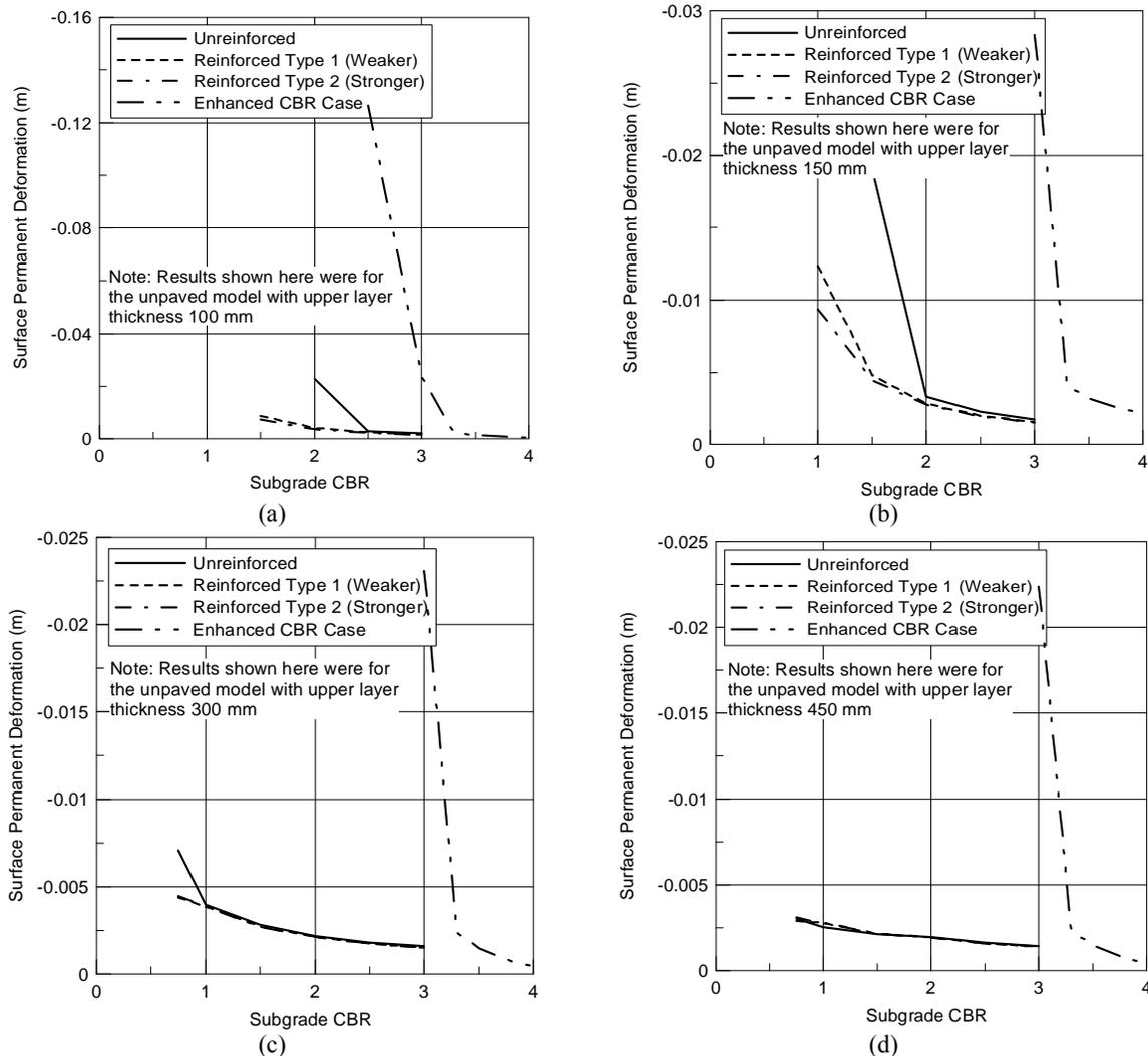
Fig. 14 Enhanced subgrade CBR analyses for different aggregate layer thicknesses
