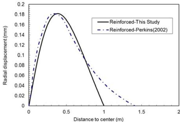
Fig. 5 Radial deformation of geogrid reinforcement
