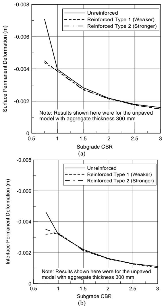
**Fig. 7** Plastic deformation V.S. subgrade CBR at (a) surface and (b) interface of a two layer system
