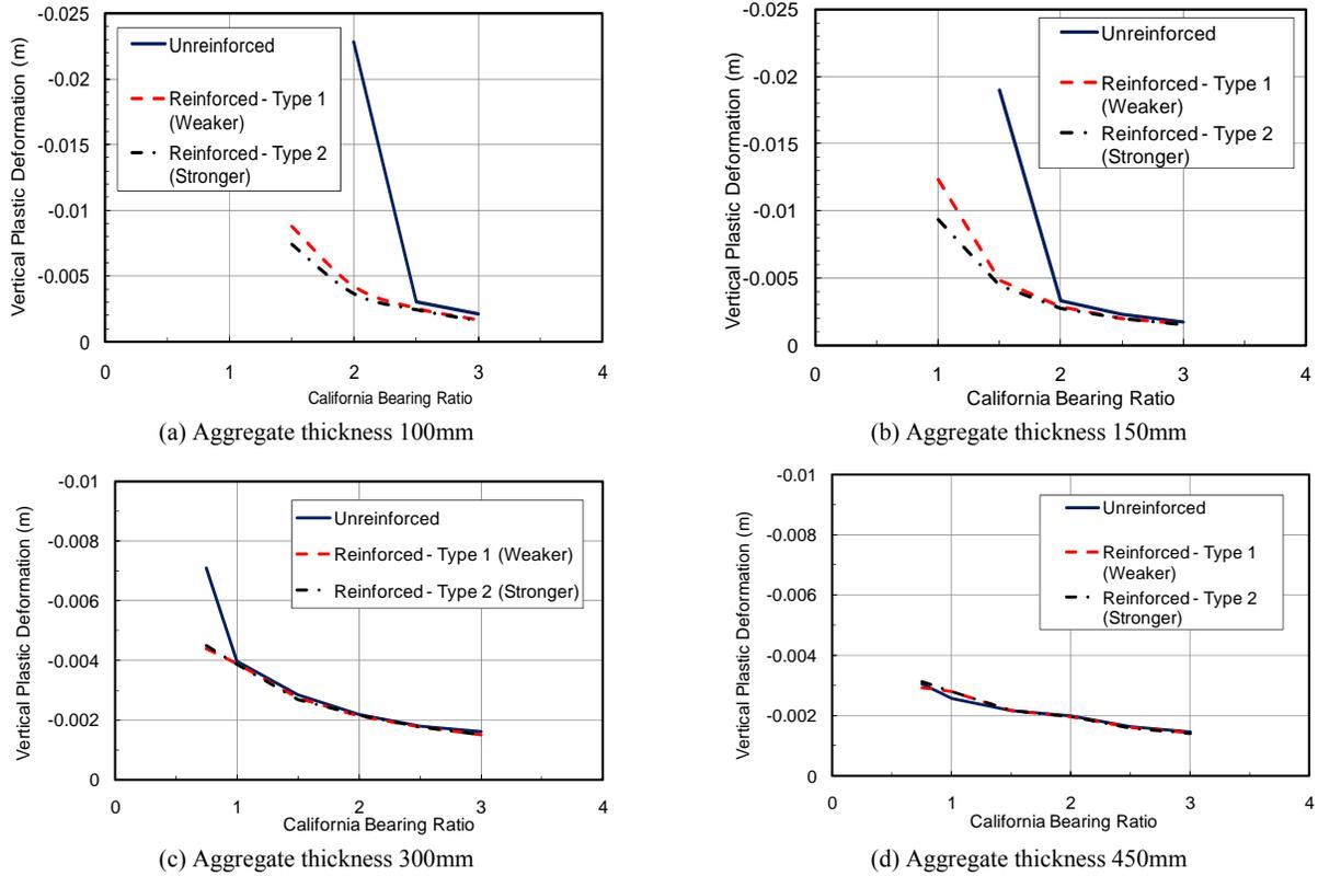
**Fig. 10** Vertical plastic deformation at the center of the loading area
