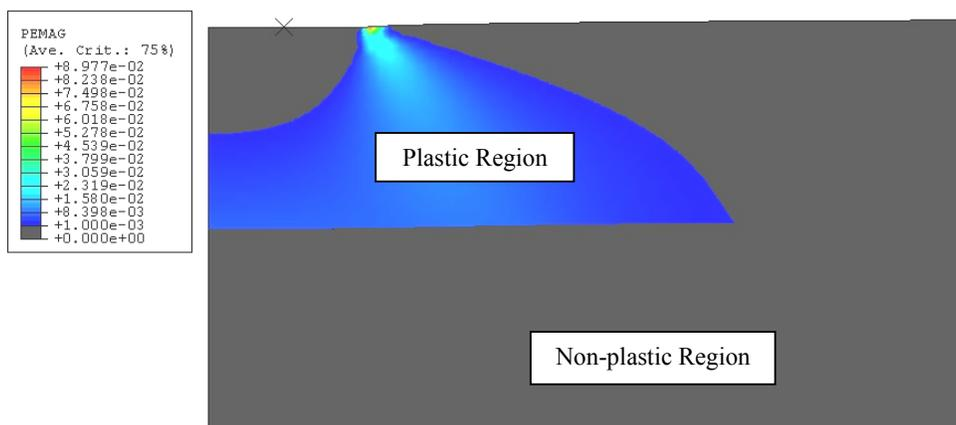
Fig. 3 Plastic region (PEMAG: the plastic strain) development in the reinforced (with geogrid) case
