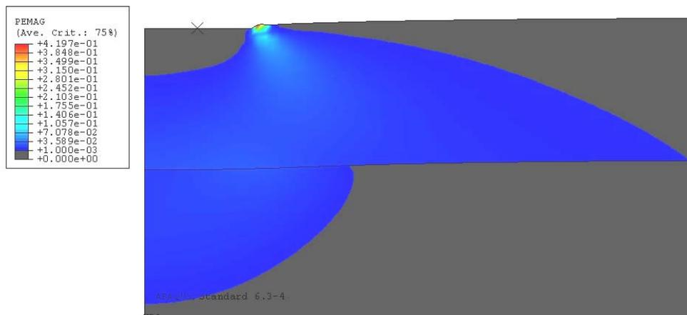
Fig. 2 Plastic region (PEMAG: the plastic strain) development in the unreinforced case
