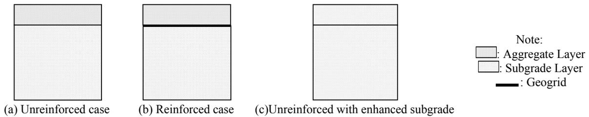
Fig. 12 Model layout for analysis of the concept of equivalent subgrade CBR
