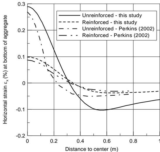
Fig. 4 Radial strain at bottom of the aggregate layer
