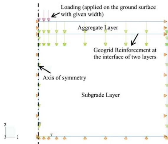
**Fig. 1** Illustration of basic numerical model with geogrid reinforcement (the arrows and triangles along the model boundary represent deformation direction and the boundary conditions)
