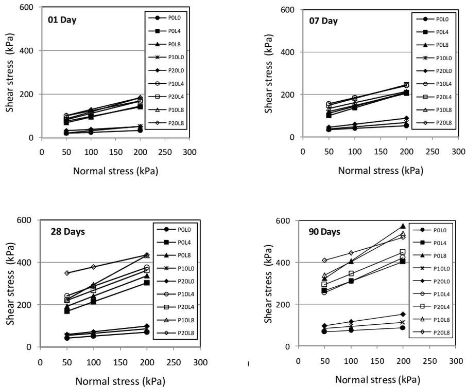
Fig. 1. Variation of shear stress with normal stress of grey soil for different curing time
