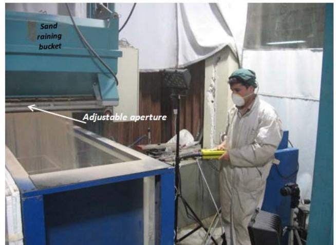
**Fig. 7** The sand raining bucket and the fault rupture box
