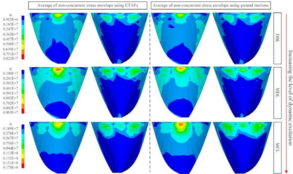
Fig. 16 Average of non-concurrent envelopes of first principal stresses on US and DS faces, (Pa)
