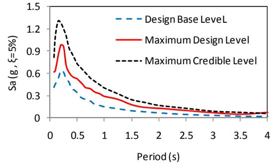
Fig. 7 Design spectrum for various performance levels in Dez Dam site
