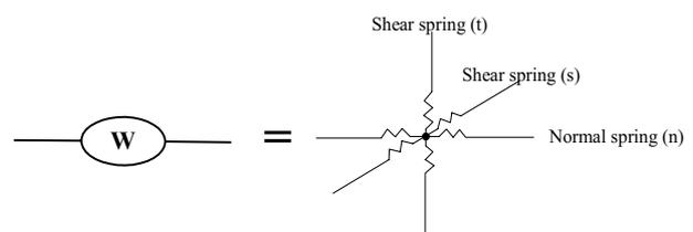
Fig. 2. Winkler spring in 3 dimensional state
