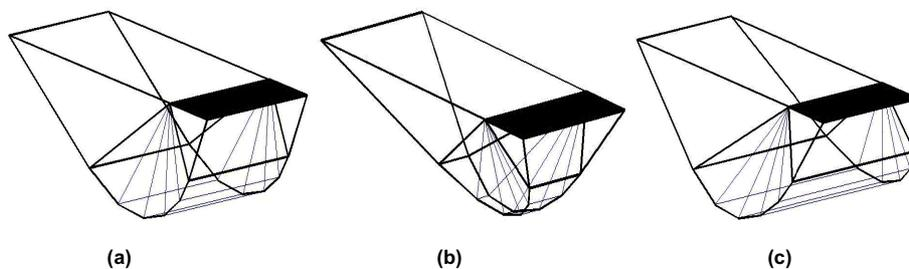
Fig. 5. The inclination of lateral failure surfaces in the three dimensional space, (a)- zero value for  $\theta_1$  and  $\theta_2$  (vertical), (b)- negative value (inclined inwards), (c)- positive value (inclined outwards).
