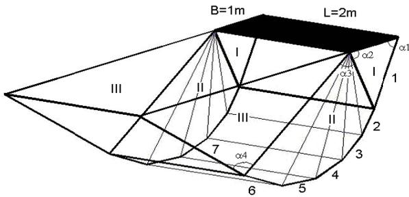
Fig. 7. Discrete element mesh for modeling progressive failure
