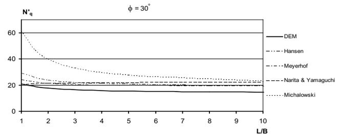
**Fig. 16.** Comparison of  $N'_q$  obtained from various methods for  $\phi = 30^\circ$
