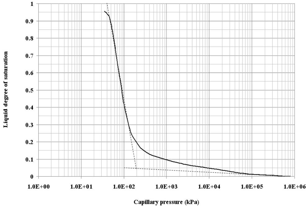
**Fig. 1** Constitutive relation between capillary pressure and liquid degree of saturation
