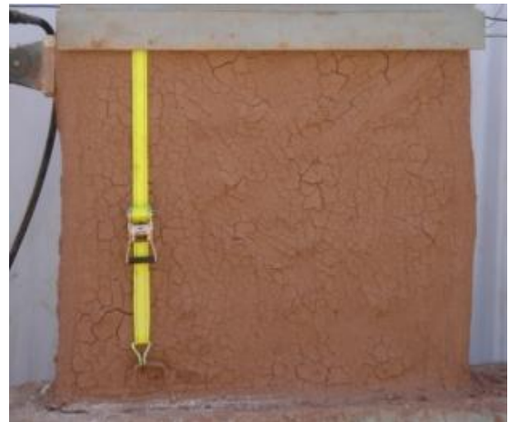
Fig. 17 Use of tarpaulin belts to prevent rocking motion mechanism
