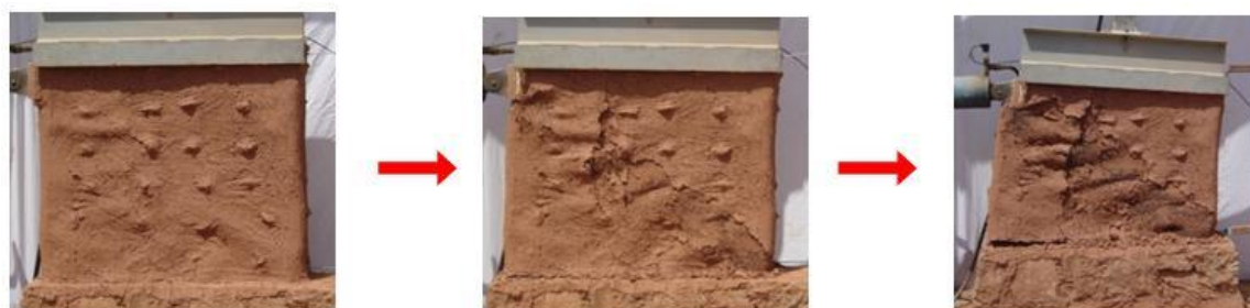
Fig. 15 Damage mechanism of RMW1 wall
