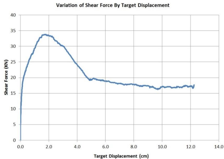
Fig. 16 Experimental behavior of RMW1 wall
