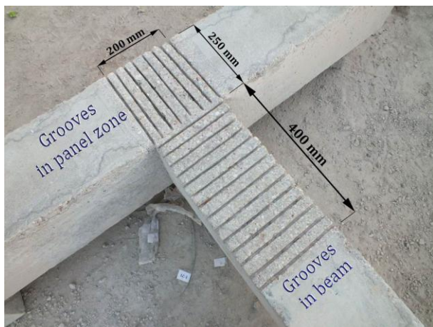
Fig. 2 Grooving pattern in specimen RW2
