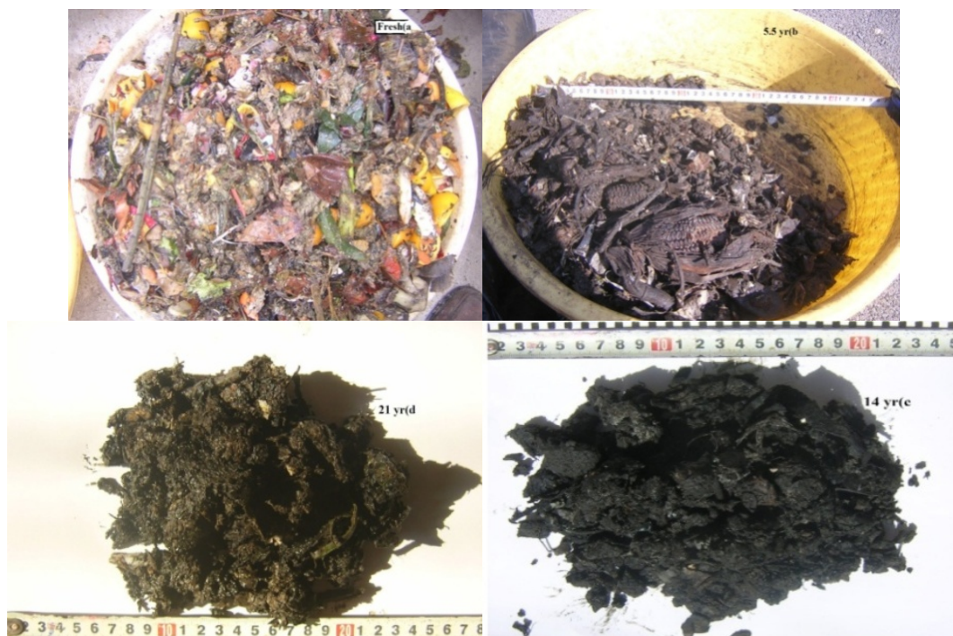
Fig. 5 Visual status of waste contribution for different samples: (a) fresh waste, (b) 5.5-year-old sample, (c) 14- year-old sample, (d) 21-year-old sample
