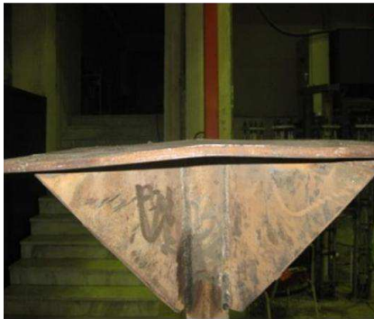
Fig. 25 Sagged plate near the connecting bolt
