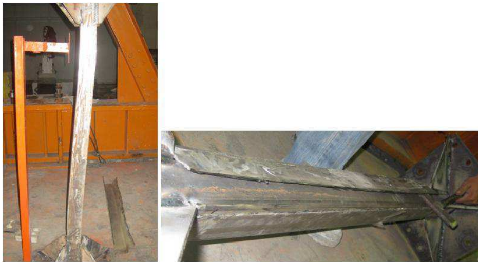
Fig. 27 Core buckling under the second mode
