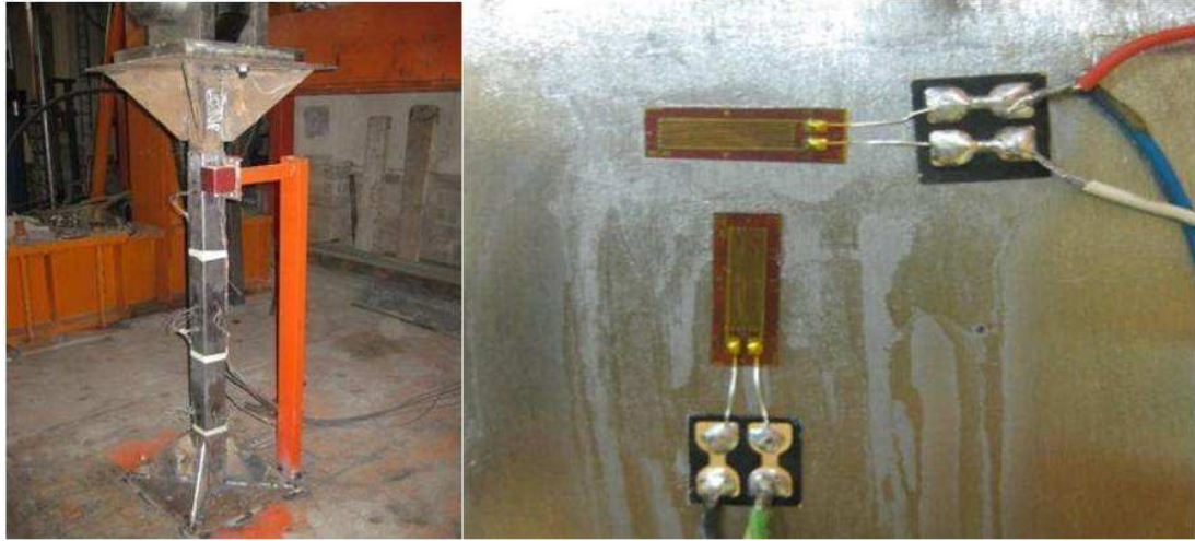
Fig. 24 Experimental set up and the position of strain gauges
