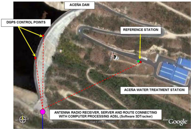
Fig. 6 DGPS spatial arrangement in La Aceña Dam
