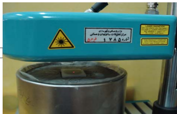
Fig. 3. Picture of test apparatus and the setup for measurement of early age shrinkage
