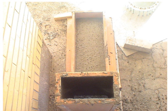
Fig. 5. L-box test of SCLWC
